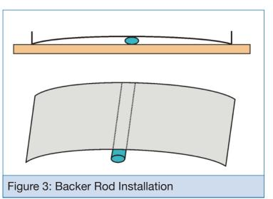
One approach for minimizing oil-canning on some profiles is to use a backer rod or some type of compressible material under
