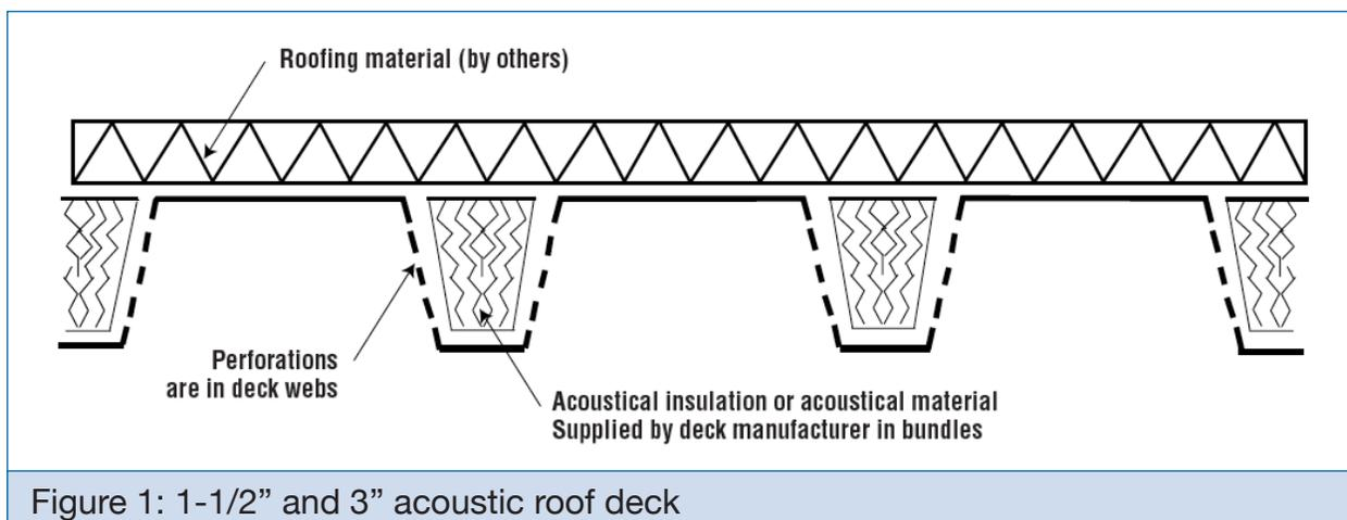
Figure 1: 1-1/2" and 3" acoustic roof deck
