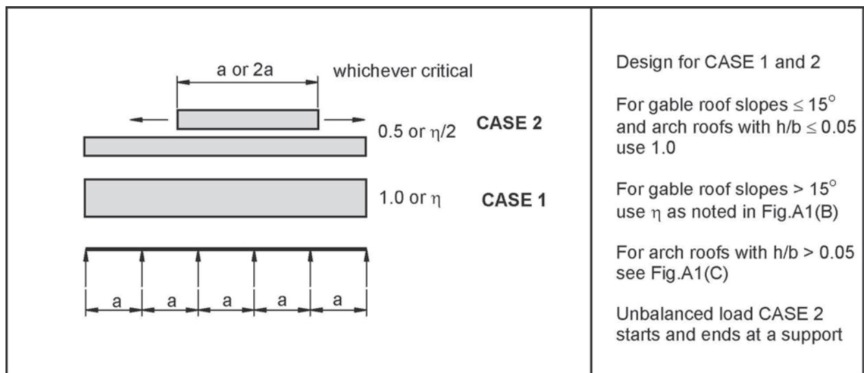
Figure 2-6: Shape Factor, C_a , for Continuous Purlins
