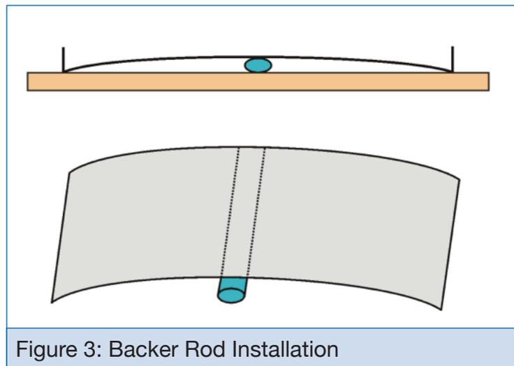
Figure 3: Backer Rod Installation
